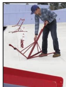
SpeedStands are engineered to be easy-to-use, and to save labor on jobs. The broad base makes the stand stable in all directions, which allows stands to be spaced 40-feet apart. The extended spacing results in fewer stands being needed for any given roof perimeter. Fewer stands reduce cost, save set-up labor, and reduce handling.
